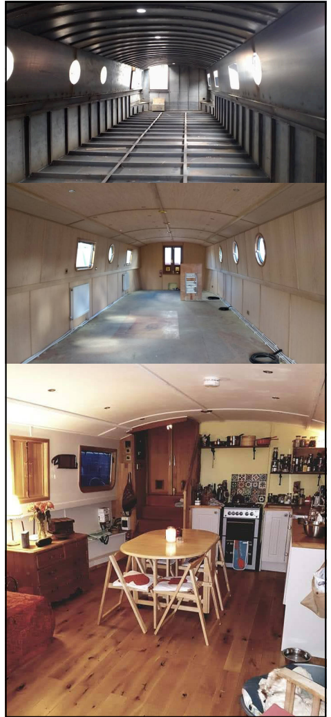
Papillon's interior unlined, lined, and completed.
